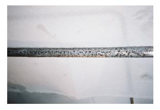
**First month inspection-** an inspection at one month shows a slight decay of the anode already present. Initial reaction is encouragement as decay is evidence that the anode is sacrificing itself to the cathode. However, the question remains. *Is the tank being protected?*
